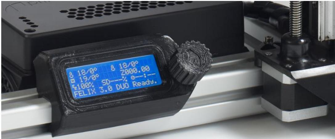
Press the rotary button to go from display mode to the top menu. A cursor indicates the current menu selection; turn the knob to move up or down, and press it to select an item.
