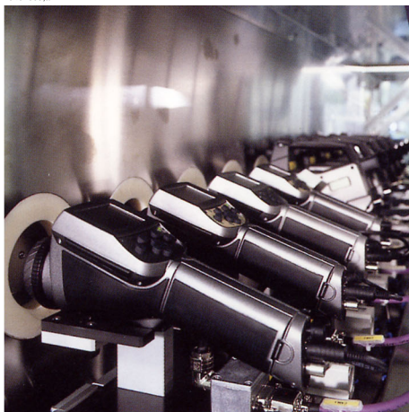
Figure 14.4 LEFT: Testing of IR cameras in the climatic chamber; RIGHT: Robot for camera testing and calibration.
