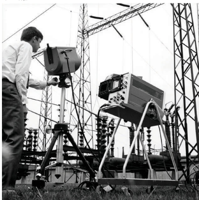
Figure 14.1 LEFT: Thermovision® Model 661 from 1969. The camera weighed approximately 25 kg (55 lb.), the oscilloscope 20 kg (44 lb.), the tripod 15 kg (33 lb.). The operator also needed a 220 VAC generator set, and a 10 L (2.6 US gallon) jar with liquid nitrogen. To the left of the oscilloscope the Polaroid attachment (6 kg/13 lb.) can be seen. RIGHT: InfraCAM from 2006. Weight: 0.55 kg (1.21 lb.), including battery.
